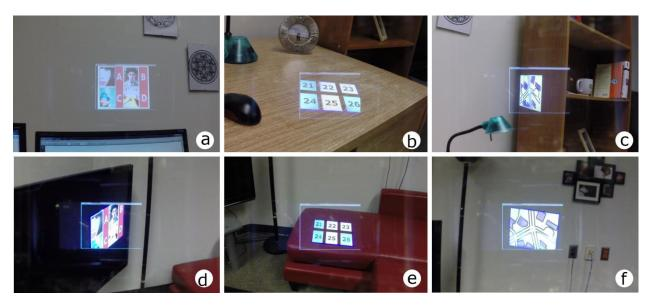
Figure 8. Images of our implementation through a Moverio BT-100 HWD showing spatially consistent layouts across office (a-c) and living room (d-f) environments. Regardless of the current location the user's applications can be found in similar relative locations. For example in this layout, the contact list (a, d) is in or above the user's forward view, the calendar (b, e) is on the lower right and a map application is on the upper right (c, f).
