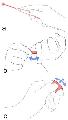
Figure 3. A variety of handheld or wearable devices can potentially be developed to provide interaction with SAIs. Possible form factors include a stylus for pointing (a), a ring for scrolling (b) or a finger pad for 2D input (c).
